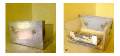
Figure 3.11: Incubator humidifier holder.
