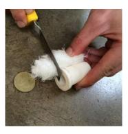
**Figure 3.18:** Creating a Gauze Filter, cutting to the right size
