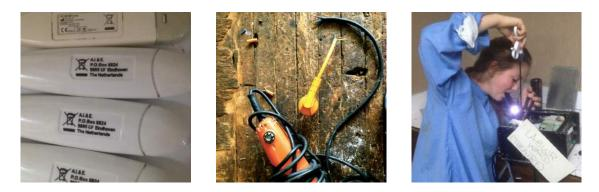
**Figure 3.3:** Left: Four broken thermometers we were given by the medical ward, which all worked after changing the batteries. Center: Cast cutter that needed a different plug. Right: Tubing often stretches and cracks over time, increasing the likelihood of leaks. Here, Ashley is repairing an automatic blood pressure monitor by replacing the old tubes with newer tubing cannibalized from an old blood pressure cuff.
