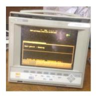
**Figure 5.1:** Cardiac monitor from the SICU and MICU. Several of these machines have been donated to KCMC. Usually the machines work, the most common problem being either the power supply, *SPO*<sub>2</sub>-meter, blood-pressure cuff or lack of ECG electrodes and ECG gel.
