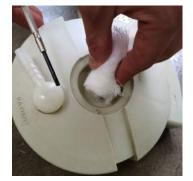
**Figure 3.20:** Placing the rolled gauze filter in place of the original filter.
