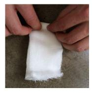
**Figure 3.19:** Creating a Gauze Filter, Rolling up the gauze filter tightly
