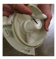
**Figure 3.21:** Placing the Gauze tightly
