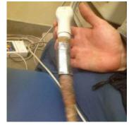
Figure 5.2: A problem commonly seen in ultrasound machines is damage from stress and strain at the junction of the cable and transducer cord.
