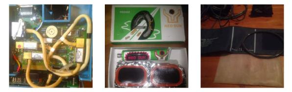
**Figure 3.1:** Aged tubing was one of the most common and simple fixes we encountered. Left: A Vital Signs Monitor, illustrating the amounts of tubing often found in medical equipment. Center: Aged rubber can simply be fixed using normal vulcanizing rubber bicycle patches. Right: A typical blood pressure cuff that can be repaired using bicycle patches as the bag is made of plastic. 5.6
